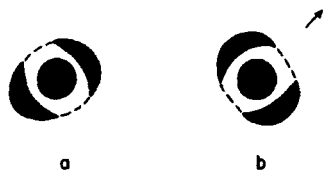
FIGURE 2 Tracings of normal-beam x-ray photographs of nematic phases. (After Kast. 27 ). a. p -azoxyanisole without a field. (Arcing is attributed to orientational effect of capillary walls). b. p -azoxyanisole aligned in an electric field (direction indicated by arrow).
